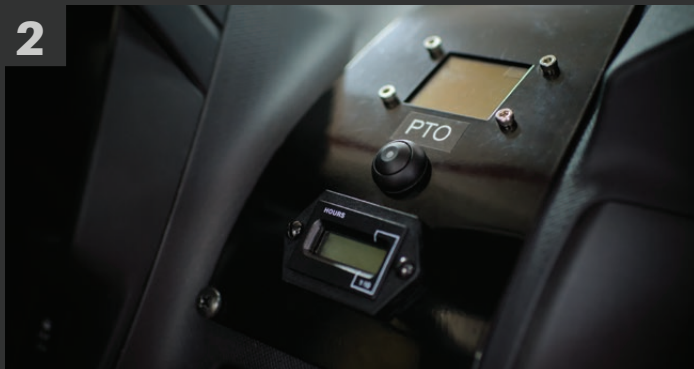
Pump controls for 70 GPM fire pump
